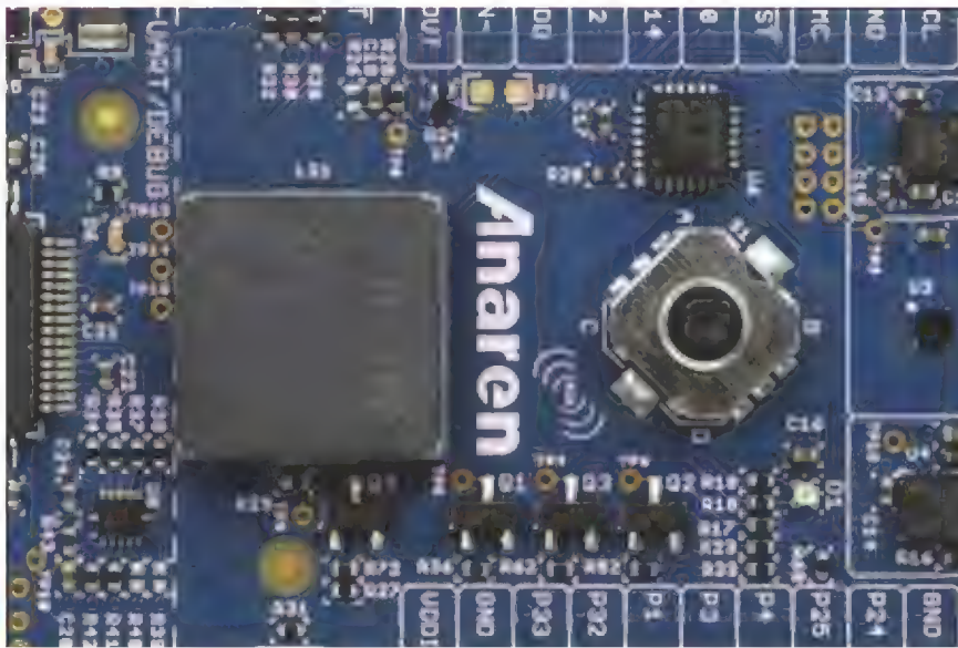
■ Photo 3. The buzzer is a real fooler. We are so used to seeing buzzers with a round housing with a center sound hole. The digital joystick you see in this shot is actually just a 4PST rotational switch (A, B, C, D) with an additional SPST switch in the push position.
